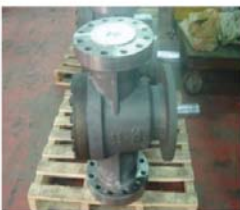
3Z Metal Seated Plug Valve, Lubricated, Full Bore Type
